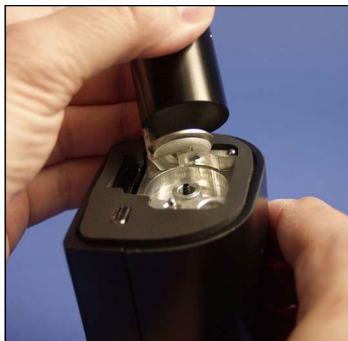
Figure 3 Installing a sample filter in the mass sensor.
