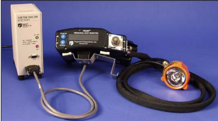
Figure 2 PDM installed on charging/communication module.
