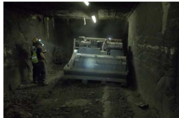
Figure 5. Asphalt Zipper Cutting the Installation Sites
