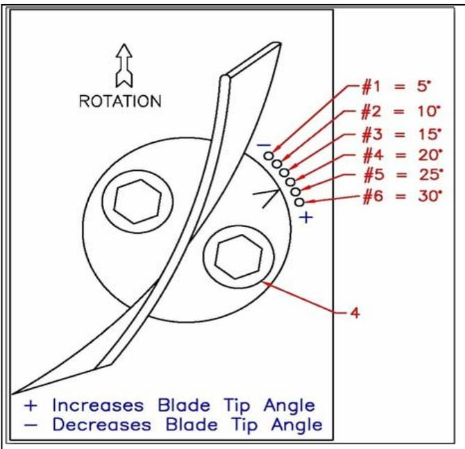
Figure 7. Manufacturer's drawing of various blade settings.
