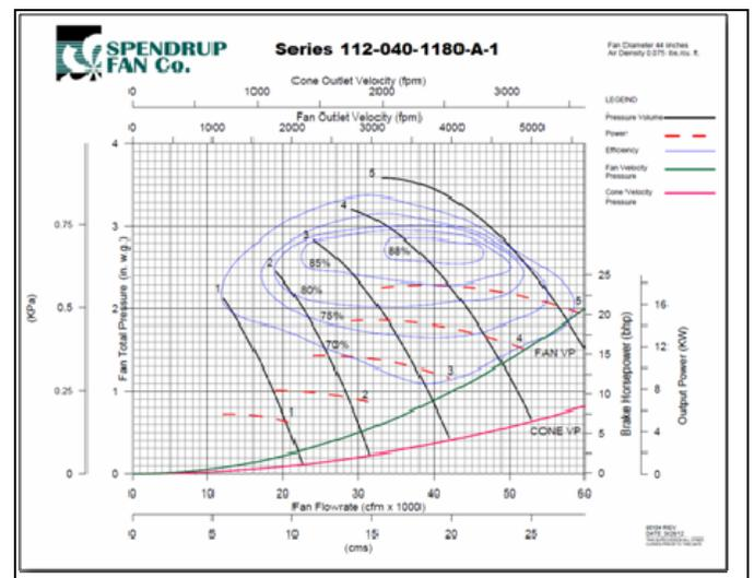
Figure 5. Booster Fan Characteristics Curve.
