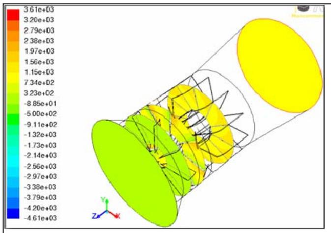
Figure 14. Total Pressure distributions (Pa) at various cross-sectional planes.
