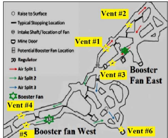
Figure 1. Missouri Experimental Mine and Booster fans location.
