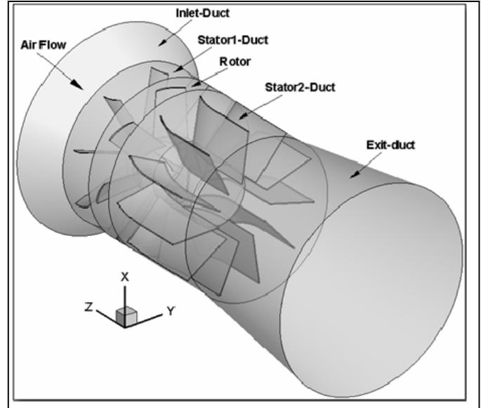
Figure 11. Fan physical model imported to Ansys Fluent.
