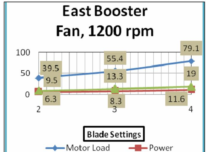
**Figure 9.** Correlation of various blade setting vs. power, current and motor load.
