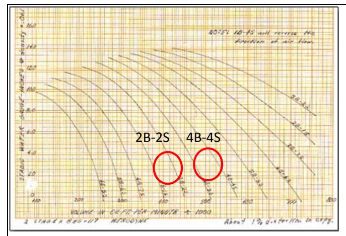
Figure 5. Main Fans Characteristics Curves.
