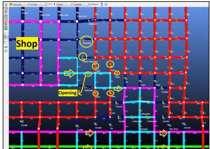
Figure 10. Scenario 2, Rerouting the Shop Air.
