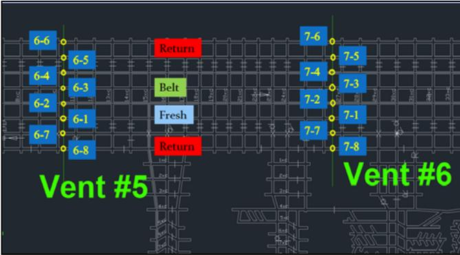
Figure 2. Example of Ventilation Stations.
