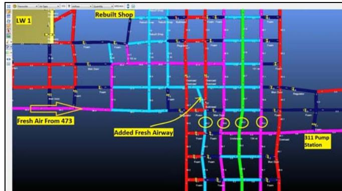
Figure 13. Scenario 5, Vetsim Visual Schematic View, Additional Fresh Airways.
