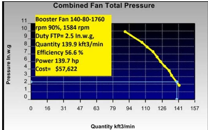
Figure 12. Scenario 3, Booster Fan Characteristics Curve.
