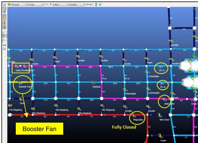
Figure 8. Additional Booster fan in Fresh Air.
