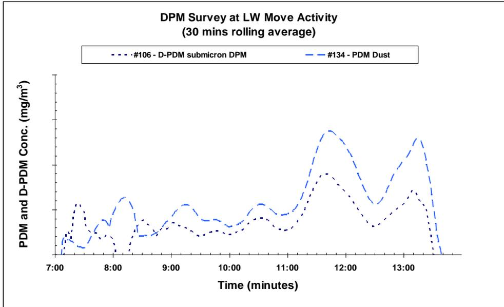
Figure 12 Monitored results with one PDM (#134) and one D-PDM (#106) side by side at a point in underground intake air in which diesel engine vehicles are operating
