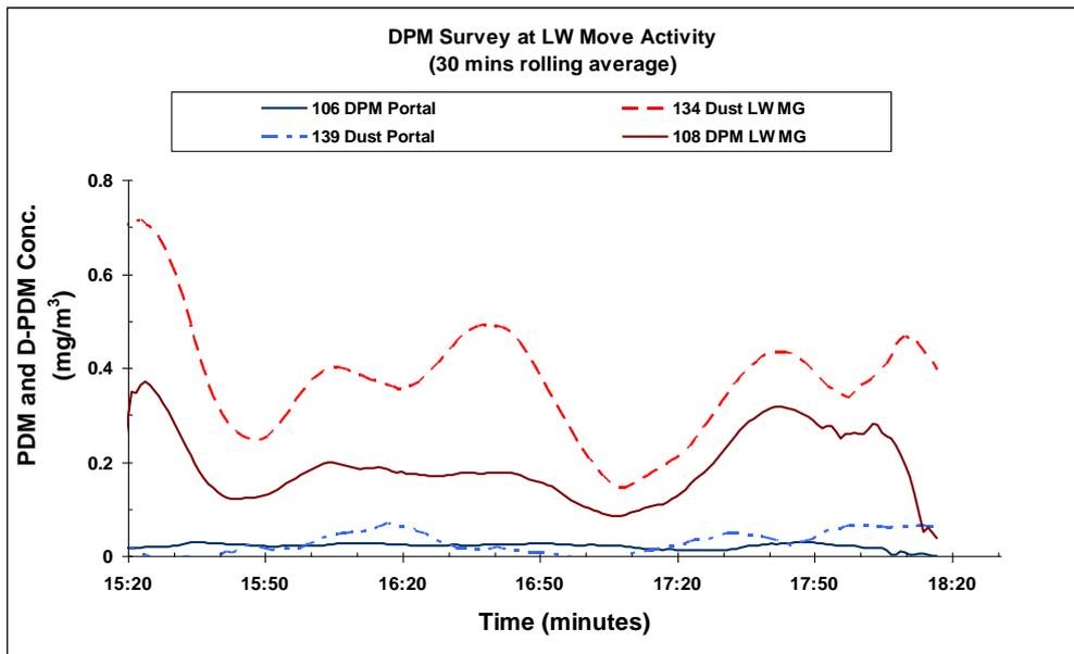
Figure 13 Monitored results with PDM (#139) and D-PDM (#106) and PDM (#134) and D-PDM (#108) side by side (upper trend lines).
