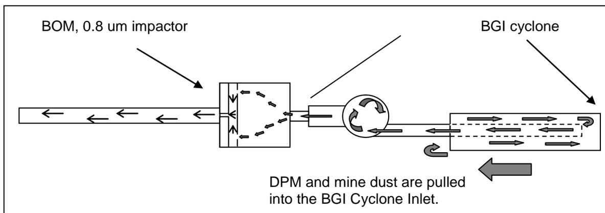
Figure 2 Schematic of prototype D-PDM Sampling Inlet.
