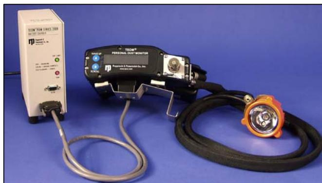
**Figure 2 PDM installed on charging/communication module.**
