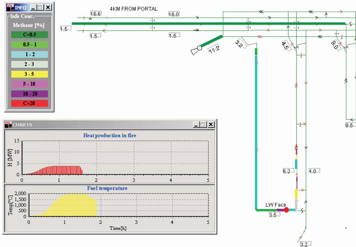
FIG 5 - Fire on gassy longwall dipping at five per cent from maingate to tailgate.
