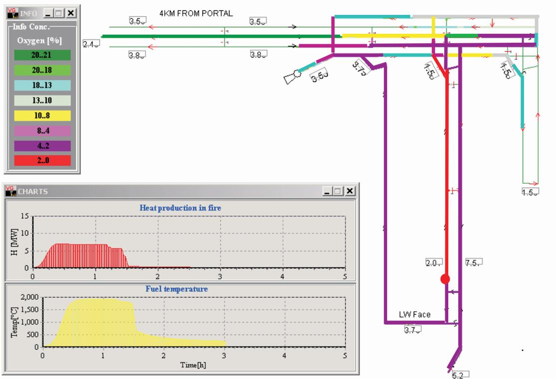
FIG 3 - GAG position at the top of back LW borehole for 4 km mains length.
