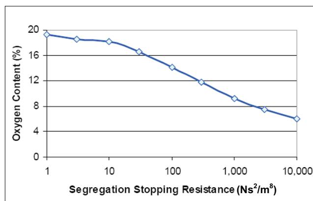
FIG 7 - Dilution of inert gas at 1.0 km from drift bottom.
