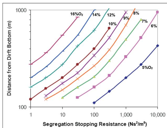
FIG 6 - Dilution of inert gas at varying segregation qualities and distance.
