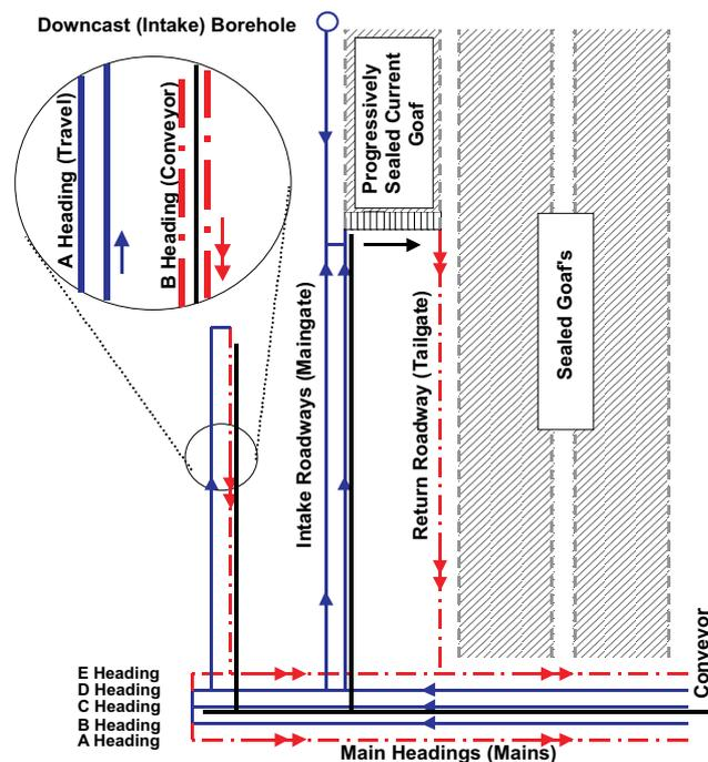
FIG 1 - Typical layout of Australian Longwall Mining.
