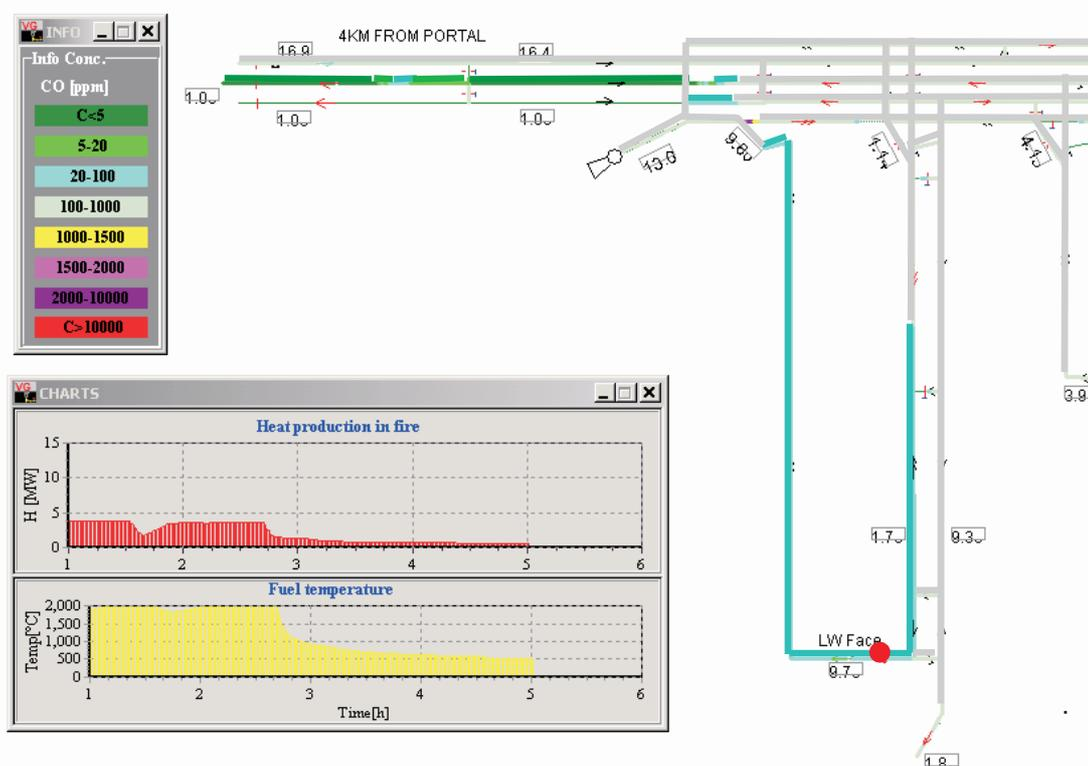
FIG 4 - Fire on gassy longwall dipping at 2.5 per cent from maingate to tailgate.
