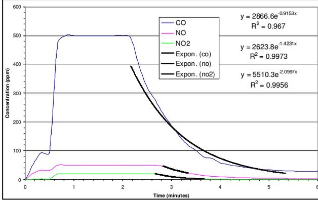
Figure 4. CO, NO and NO<sub>2</sub> readings versus time after blast.
