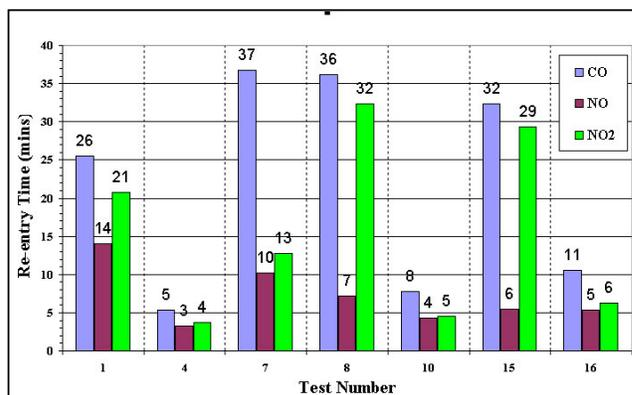
Figure 2. Re-entry times for seven development heading tests.
