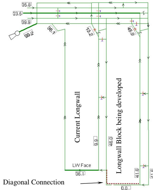
Figure 7. A typical diagonal connection in Australian coal mine.
