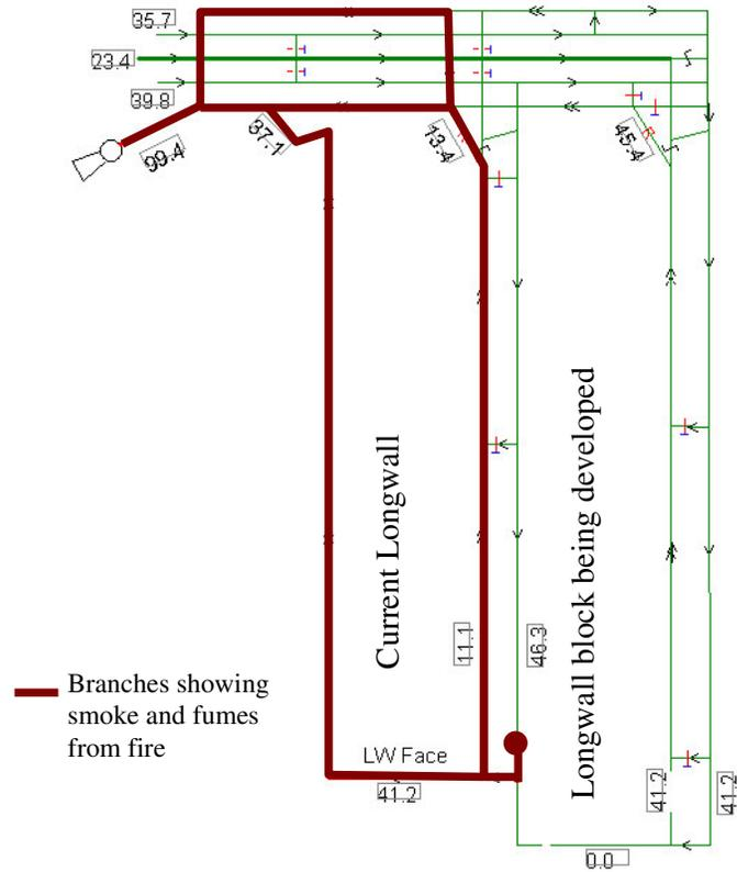
Figure 8. Smoke progression without diagonal connection.
