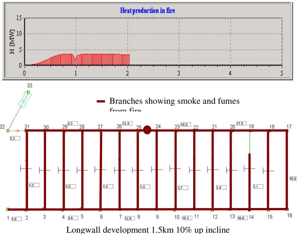
Figure 4. Smoke reversal and heat reduction observed during simulation for 10m long fire zone in return roadway.
