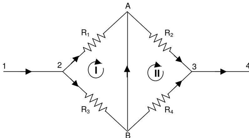
Figure 6. Ventilation network circuit - Wheatstone bridge.
