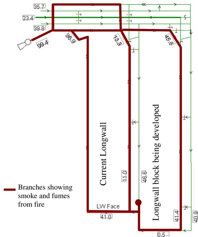
Figure 9. Smoke progression with diagonal connection.
