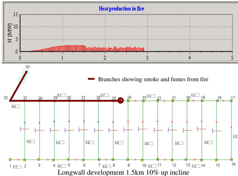
Figure 3. Smoke progressions and heat production during simulation for 5 m long fire zone in return roadway.
