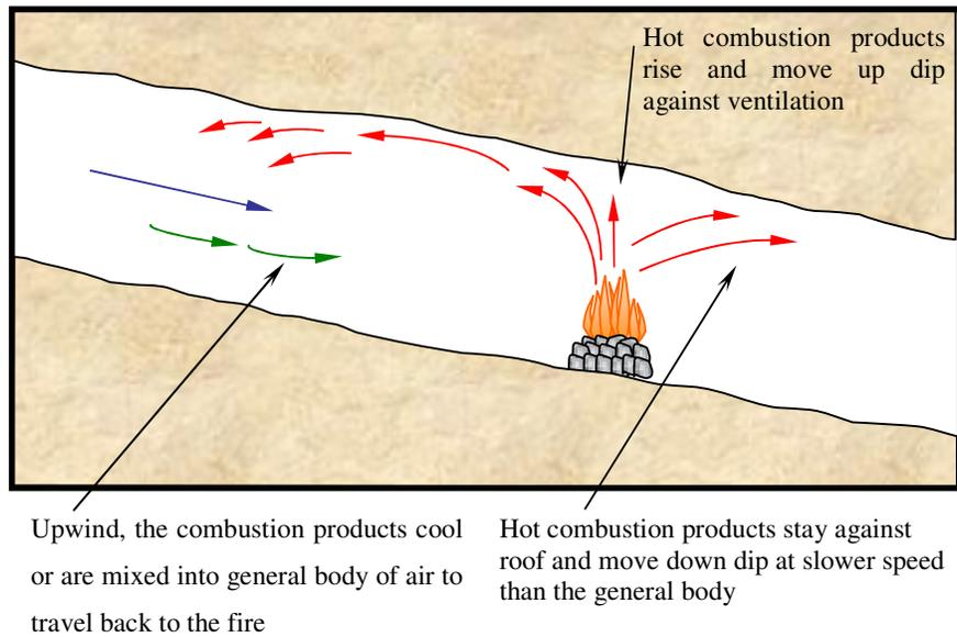
Figure 1. Buoyancy effect of fires in descental airway (after Bofinger, 1998).
