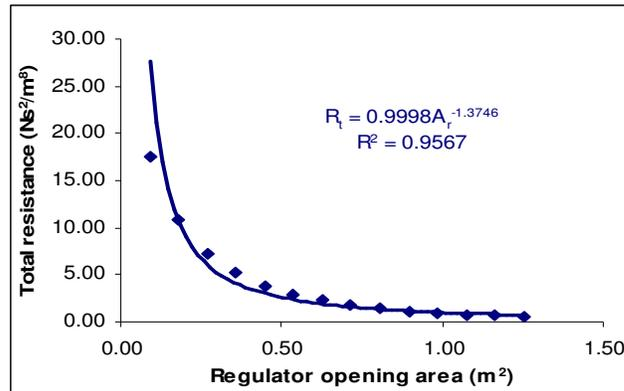
Figure 3. Relationship between new total resistance and regulator opening area.
