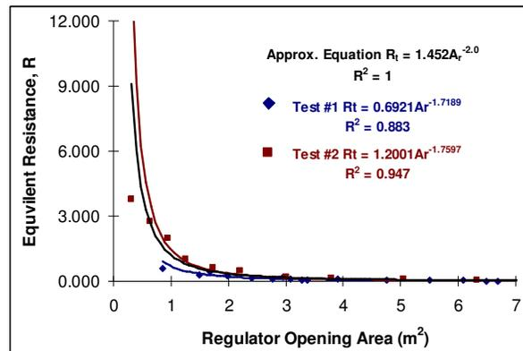
Figure 8 Relationship between resistance and equivalent opening area for louvre regulator.
