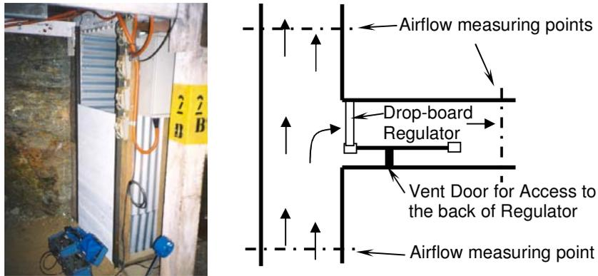
Figure 2. Drop board regulator tested at UQEM.
