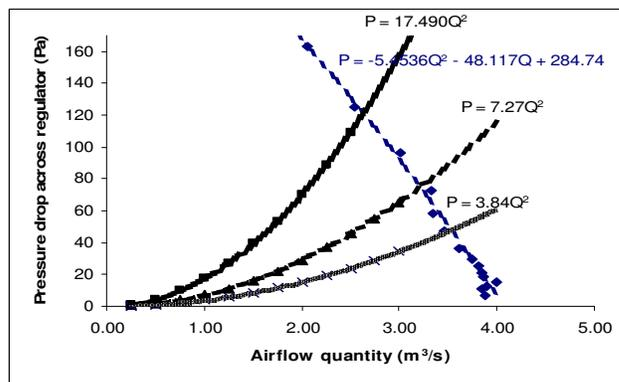
Figure 4. Drop board regulator characteristic curves.
