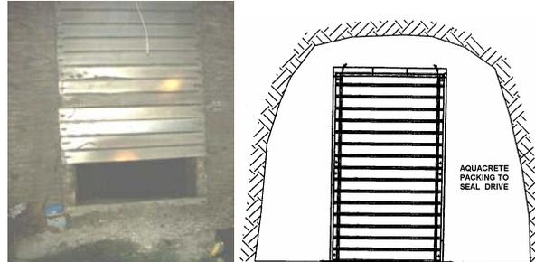
Figure 5 Photographic views and engineering drawing of a half size C-section regulator.
