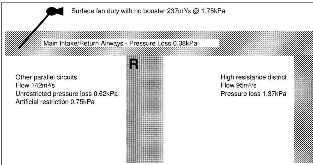
Figure 2. Longwall ventilation scheme with artificial restrictions.
