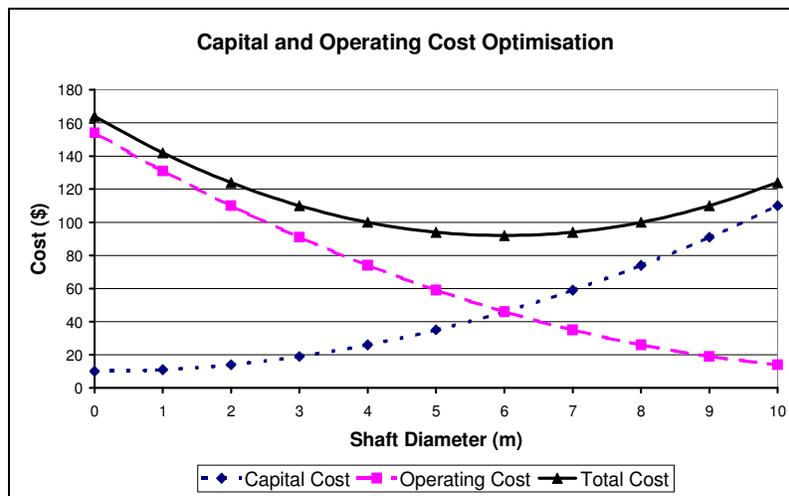
Figure 1. Theoretical example capital and operating cost function optimisation with minimum total cost indicating optimum selection of shaft diameter.
