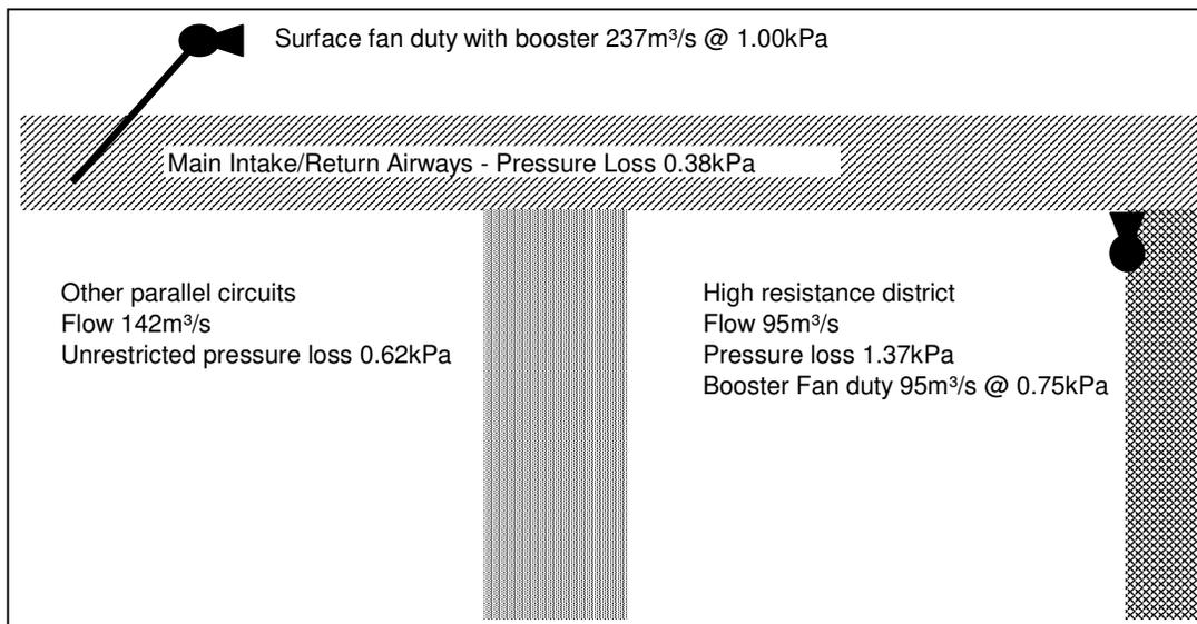
Figure 3. Longwall ventilation scheme with booster fan installed.
