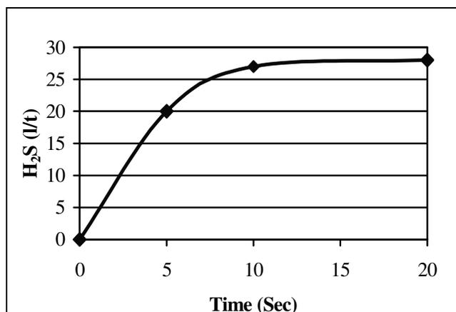
Figure 4. H<sub>2</sub>S release rate vs pulverising time
