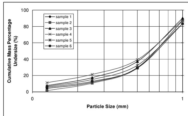
Figure 10. Trend of % weight undersize vs particle size
