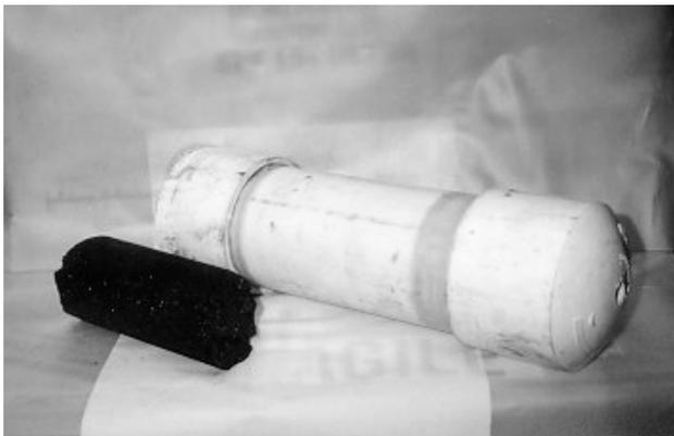
Figure 1. Core sample and plastic pipe container
