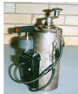
Figure 3. Drum tumbler system and portable gas analyser
