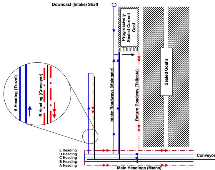
Figure 1. Typical Layout Aspects of Australian Longwall Mining
