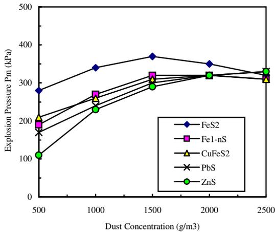
**Figure 2 Explosion Pressure P<sub>m</sub> of the Concentrated Sulphide Minerals**
