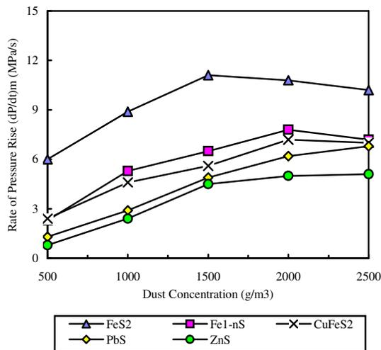
**Figure 3 Rate of Pressure Rise (dP/dt)<sub>m</sub> of the Concentrated Sulphide Minerals**
