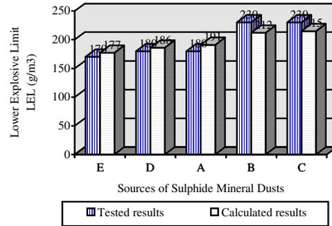
**Figure 8 Comparison of Tested and Calculated LELs for the Sulphide Dusts**
