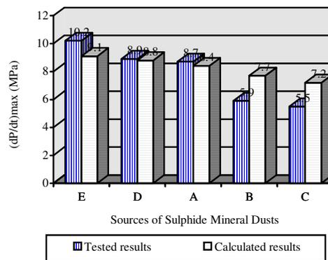
**Figure 10 Comparison of Tested and Calculated  $(dP/dt)_{max}$  for the Sulphide Dusts**
