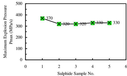
**Figure 4 Maximum Explosion Pressure of Concentrated Sulphide Minerals (Sample No.: 1 - FeS<sub>2</sub> concentrate, 2 - Fe<sub>1-n</sub>S concentrate, 3 - CuFeS<sub>2</sub> concentrate, 4 - PbS concentrate, 5 - ZnS concentrate)**
