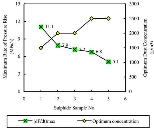
**Figure 5 Maximum Rate of Pressure Rise of Concentrated Sulphide Minerals (Sample No.: 1 - FeS<sub>2</sub> concentrate, 2 - Fe<sub>1-n</sub>S concentrate, 3 - CuFeS<sub>2</sub> concentrate, 4 - PbS concentrate, 5 - ZnS concentrate)**
