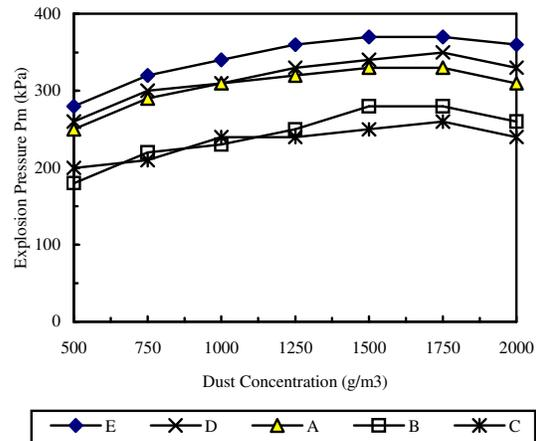
**Figure 6 Explosion Pressure  $P_m$  of Sulphide Dust Samples**
