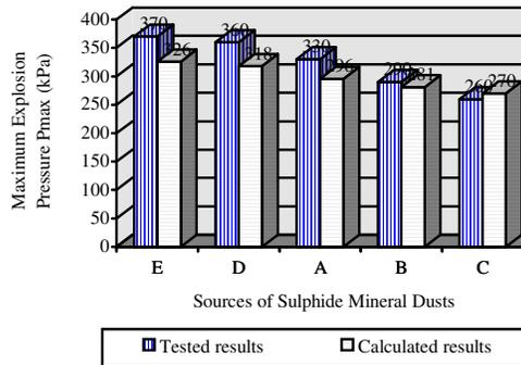
**Figure 9 Comparison of Tested and Calculated  $P_{max}$  for the Sulphide Dust Samples**
