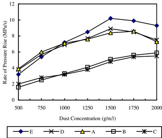
**Figure 7 Rate of Pressure Rise  $(dP/dt)_m$  of Sulphide Dust Samples**
