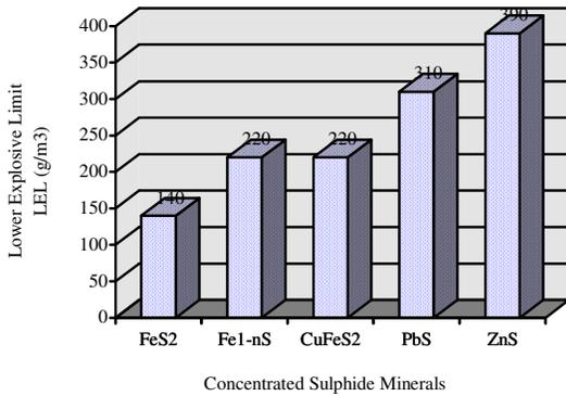
**Figure 1 Lower Explosive limit of Concentrated Sulphide Minerals**
