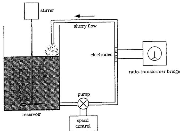
FIG 2 - Slurry concentration measurement pilot plant.
