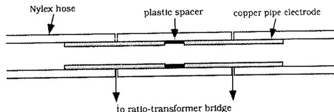
FIG 3 - Pilot plant electrode section.
