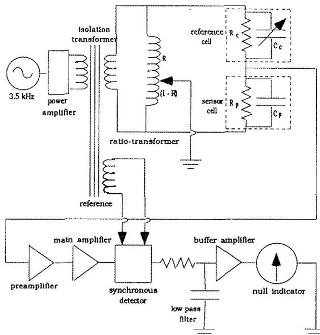
FIG 1 - Schematic of the ratio-transformer bridge modified for resistance measurement of coal slurry solids concentration.
