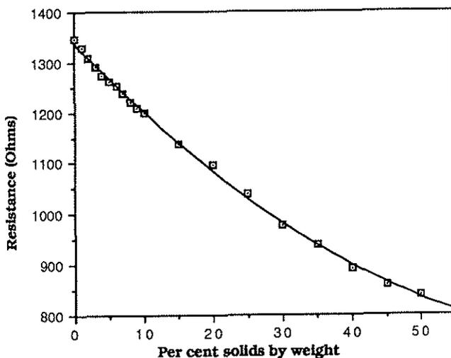
FIG 4 - Graph of coal slurry resistance against concentration.
