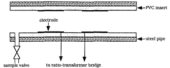
FIG 5 - Tailings pipe electrode test section.
