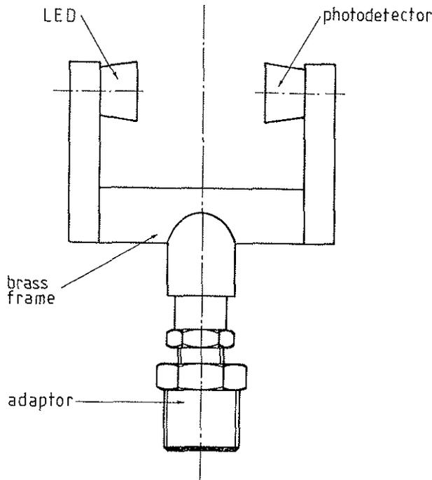
Figure 2 - Optical Dust Probe
