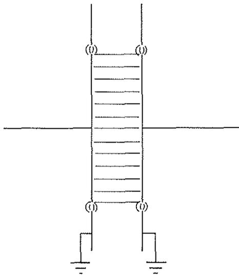
FIGURE 4(b) ELECTRIC FIELD WITH GUARD ELECTRODES
