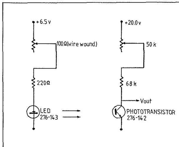
Figure 3 - Circuit Diagram of the Dust Concentration Probe
