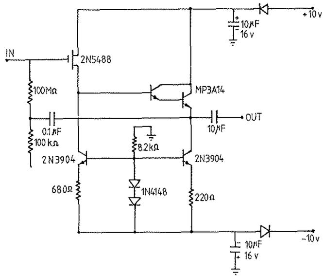
Figure 8 - 50 MΩ Preamplifier
