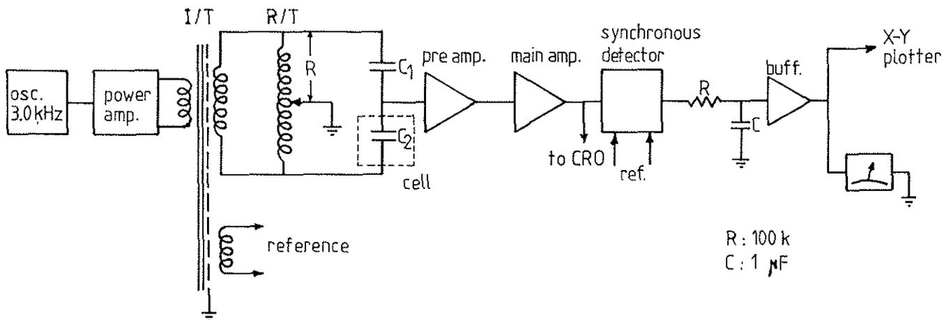
Figure 7 - Schematic of Cell and Electronic Circuitry
