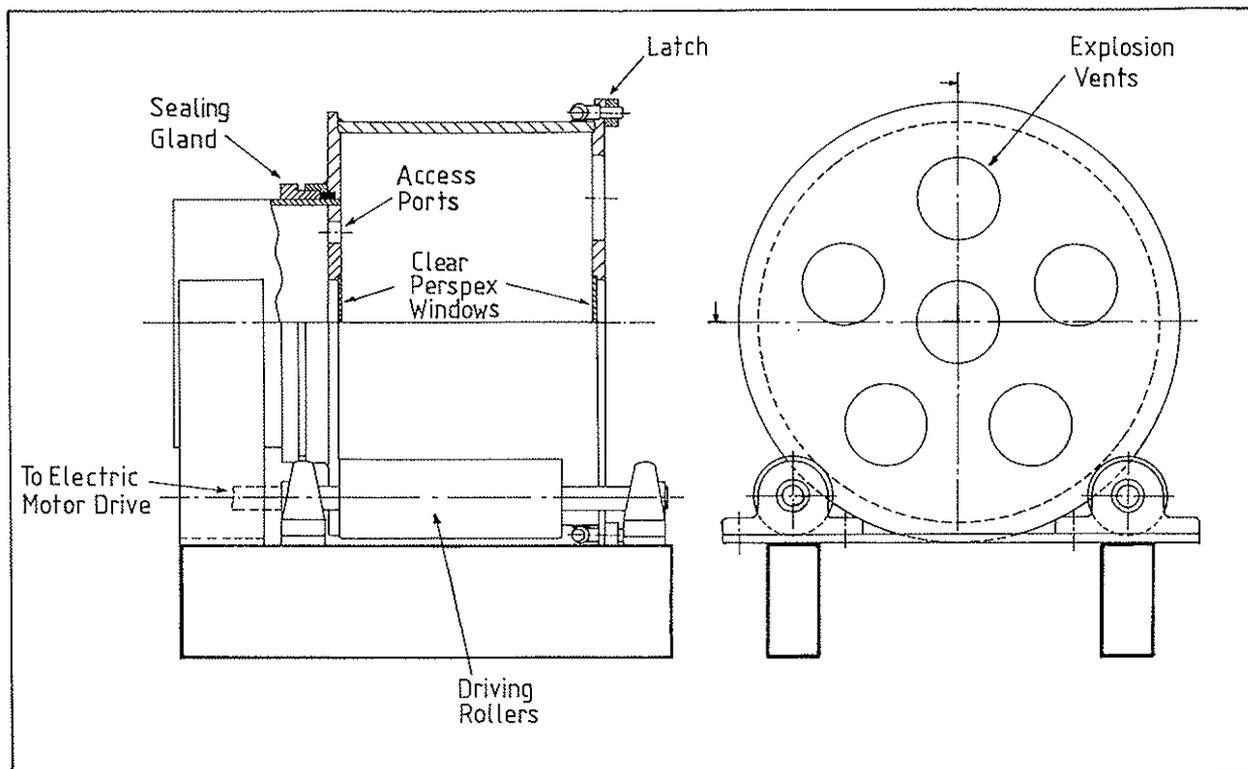
Figure 1 - Explosion Chamber
