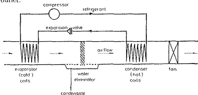
Fig. 1—Diagrammatic representation of cooler/dehumidifier/heater unit
