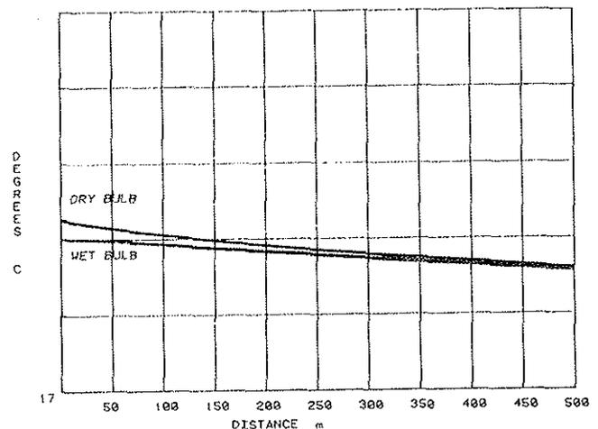
Fig. 2—Computer simulation of wet and dry bulb temperatures before the dehumidifier unit is installed (condensation throughout).
