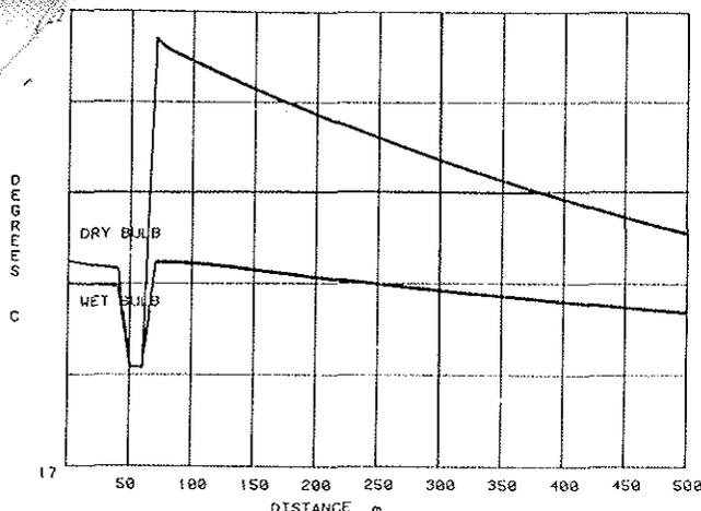
Fig. 3—Computer simulation of wet and dry bulb temperatures with dehumidifier at 40-60 m (131-197 ft). Airway is maintained free of condensation.
