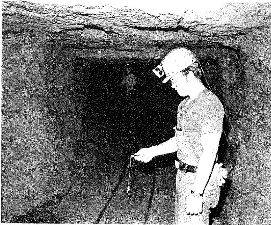
Figure 5. Sling psychrometer measuring air temperature.
