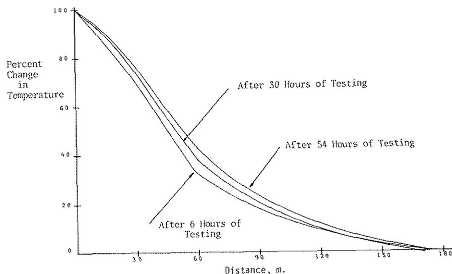
**Figure 8.** Plot of percentage change in air temperature between intake and outlet airway points at distances from intake portal.
