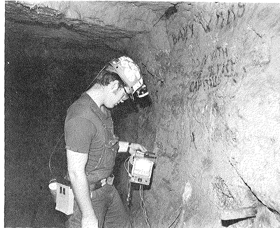
Figure 4. Telethermometer for measuring rock temperature.
