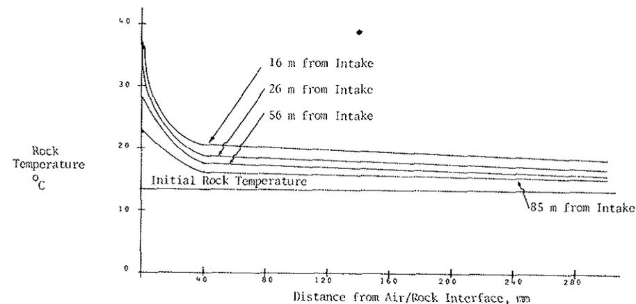
**Figure 9.** Plot of rock temperature at distance from air/rock interface after 54 hours of continuous airflow.
