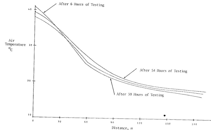
Figure 7. Plot of air temperature at distance from intake portal after 6, 30, and 54 hours of continuous airflow.
