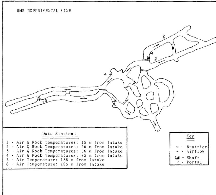
Figure 1. Plan of experimental mine.
