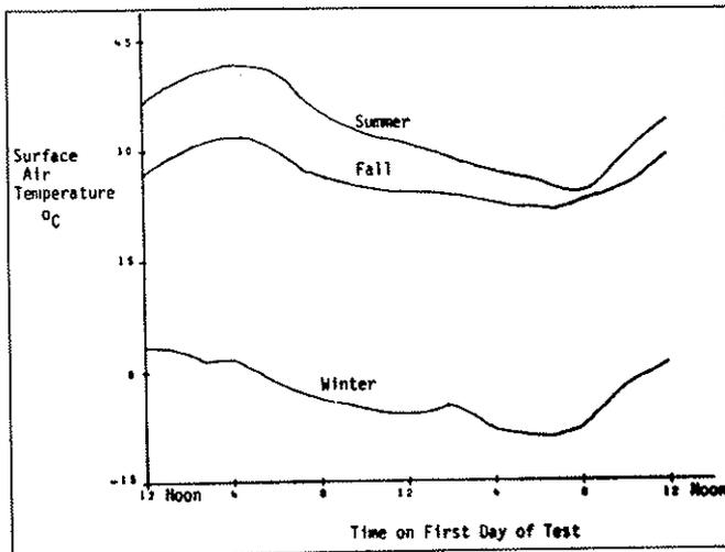
Fig. 4. Surface air temperature patterns on first day of summer, fall, and winter tests.
