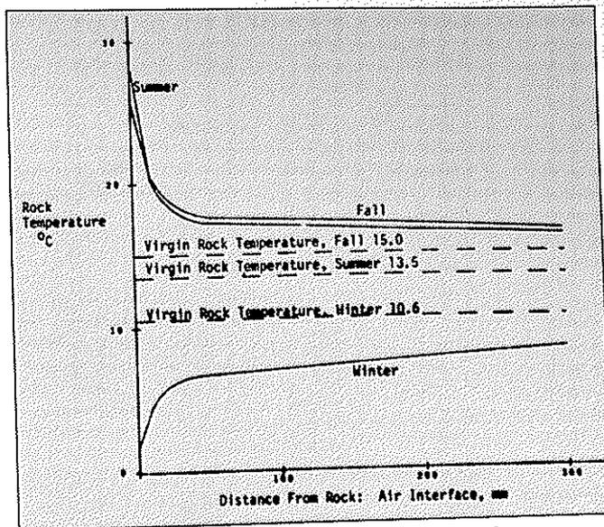
Fig. 7. Rock temperature at depth from rock/air interface.
