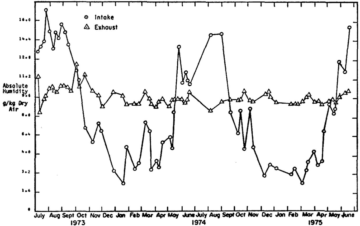
Fig. 3. Seasonal plots comparing absolute humidity at mine intake and exhaust stations (after Bruzewski and Aughenbaugh).
