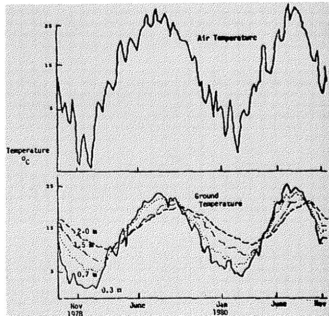
Fig. 1. Average daily temperatures, Rolla, Missouri. Air temperature and ground temperatures at depth.
