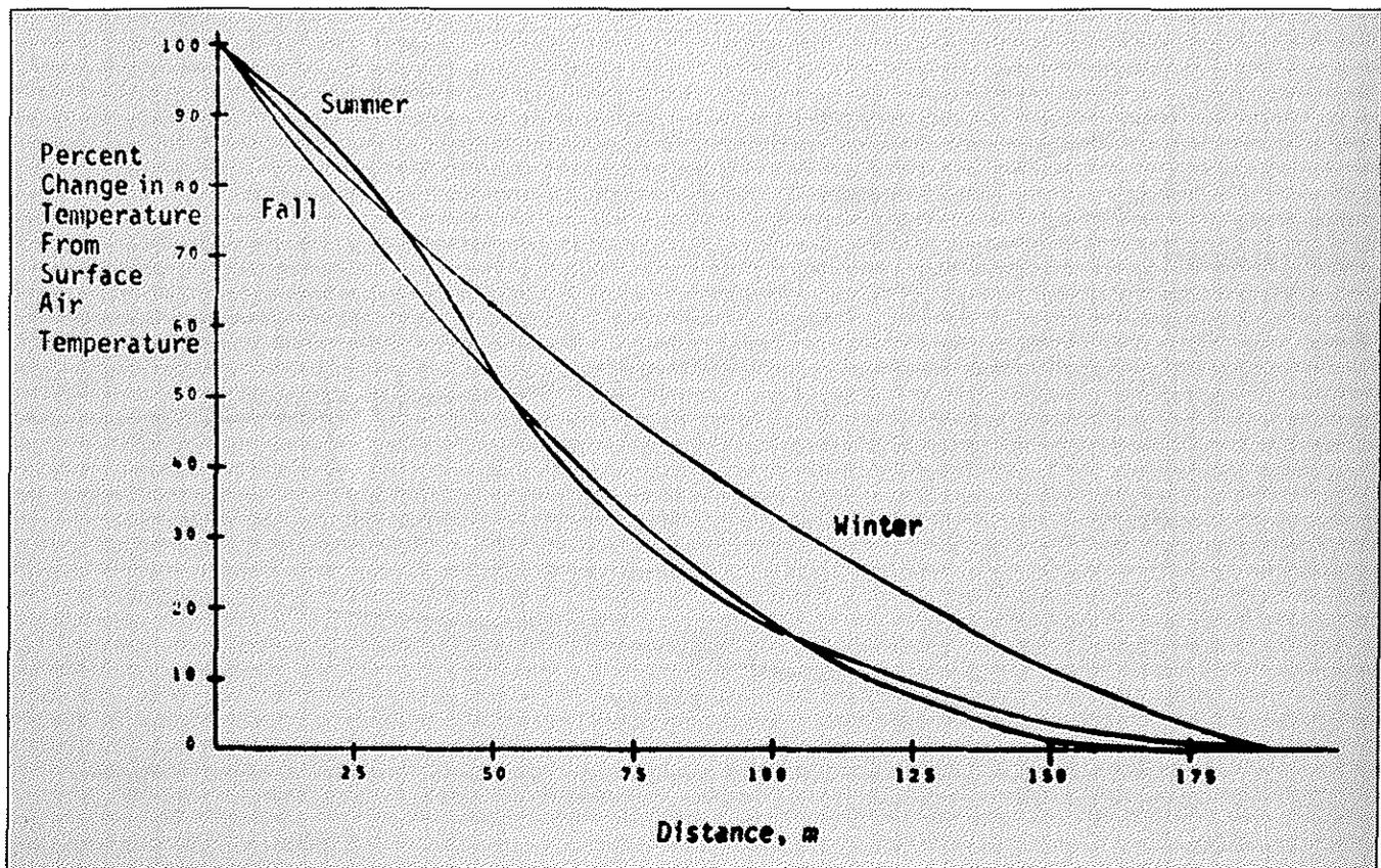
Fig. 6. Percentage change in air temperature between intake and outlet airway points against distance along passageway.
