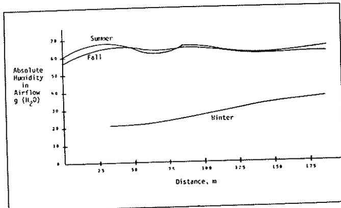
Fig. 8. Humidity levels in air flowing along passageway, mid-afternoon readings.
