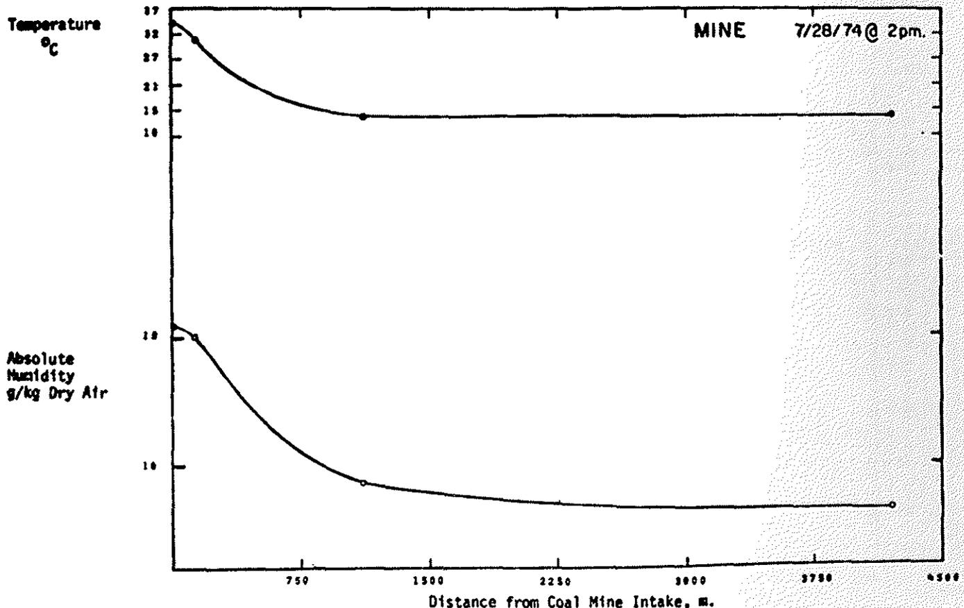
Fig. 2. Tempering of air with distance from mine surface intake portal (after Bruzewski and Aughenbaugh).
